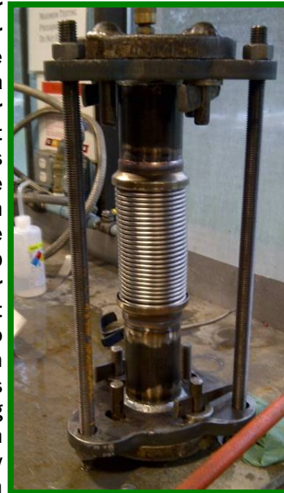
Type 311 expansion joint undergoing validation pressure testing for use with solar collector tubes.
